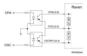
Figure 4-1: CFM and CGC Remote Control
